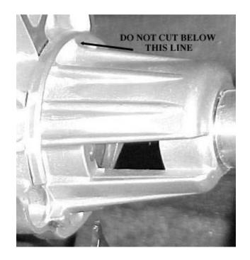
Disassemble the starter and remove the front of the gear reduction housing.
