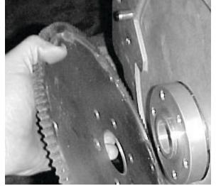
7. CAREFULLY ALIGN THE HUB SPACER/FLEX PLATE AND THE CRANKSHAFT BOLT HOLES WHILE PLACING THE HUB SPACER ONTO THE CRANKSHAFT. THE HUB SPACER SHOULD BE A CLOSE FIT TO THE
