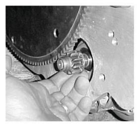
16. BEFORE INSTALLING THE TRANSMISSION, CHECK THAT THE TORQUE CONVERTER IS FULLY SEATED INTO THE FRONT PUMP OF THE TRANSMISSION. THE TORQUE CONVERTER MATING BOSSES SHOULD BE APPROXIMENTLY 1" FROM THE BELLHOUSING FACE.
